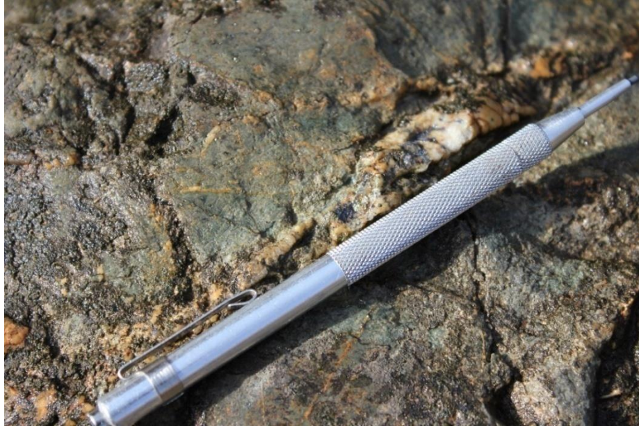
Figure 20. Molybdenite within the quartz-sulfide vein.
