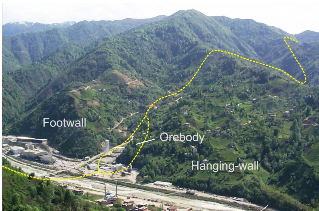
Figure 2. View to the Çayeli Cu-Zn deposit, facing W-SW. Massive ore is located between hanging-wall and footwall lithologies, but an exact location is unavailable. The footwall lithologies consist of felsic and mafic rocks. Hanging-wall lithologies mainly consist of basalt/andesite and related fragmental rocks.
