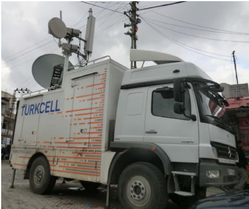
Figure 9.14. A view of a mobile telecommunication unit of TÜRKCELL in Erciş.
