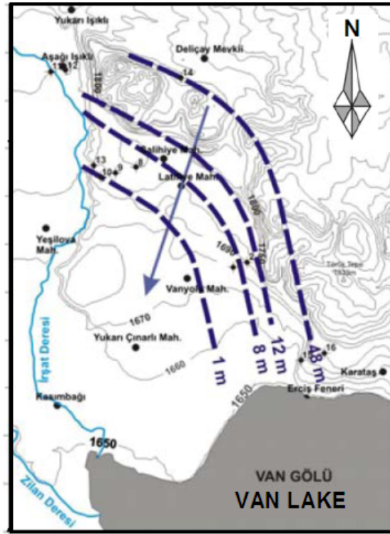
Figure 2.10. Groundwater depth contour map of Erciş town (Özvan et al., 2008)
